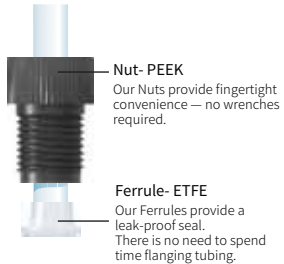
WD06B-5/16-24-K-black PEEK Flangeless Nut YK-048-F ETFE Ferrule For 4.8mm O tube
