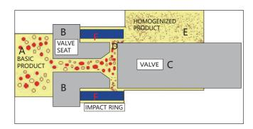
the valve at a very fast speed, resulting in cavitation effect, impact effect and shear effect, so that the aggregated material is evenly dispersed.
